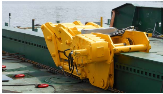
Figure 4. Shuttle System, previous handling and launching system
